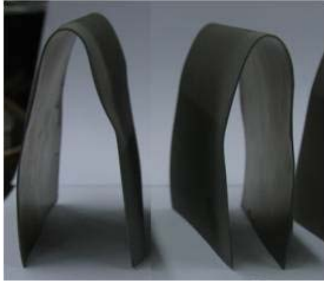
Figure 3 Severely deformed titanium leading edge sections
