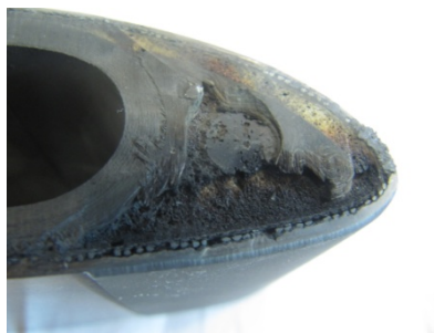
Figure 8 Initial trial of applying HVOF WC-Co to the UH-60 rotor blade section. The surface temperature was recorded at over 500F.
